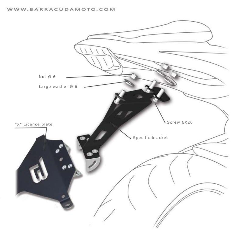
REMOVE THE ORIGINAL LICENCE PLATE FROM MOTORBIKE. APPLY THE BARRACUDA LICENCE PLATE FIXING IT WITH THE 6X20 SCREWS AND WITH THE LOCKING NUTS LIKE THE PICTURE. APPROACH AND LOCK THE "X" LICENCE PLATE TO THE BRACKET INSTALLED.
